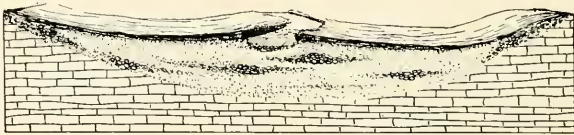
FIG. 8. Diagram showing natural levees.
